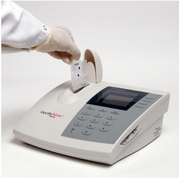
1. Open the cover and insert the test device
