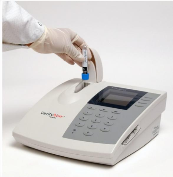
2. Insert the whole blood patient sample tube onto the assay device needle
