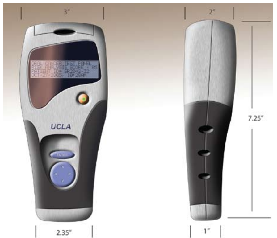
The Oral Fluid NanoSensor Test is a handheld, automated, integrated micro-electromechanical system that will enable simultaneous and rapid detection of multiple salivary protein and nucleic acid targets. The device was developed by a team of researchers at the UCLA School of Dentistry led by David Wong, DMD, DMSc.
